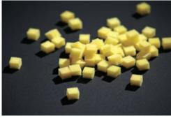
It can be fixed microorganisms in high concentration because the main material is ether based polyurethane and it is strong to hydrophilic biological affinity. In addition, the specific surface areas become larger than conventional ones.
